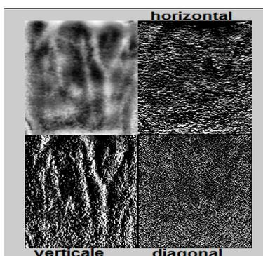
Fig (6): Discrete Bi-orthogonal wavelets transform
