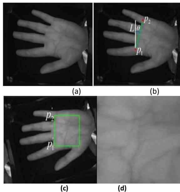
Fig. 3. Illustrations of palm vein ROI extraction (a): original hand image, (b): the angle  $\vartheta$  between line  $p_1 p_2$  and vertical line  $L$ , (c): normalized palm vein image, and (d): palm vein ROI.
