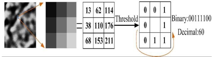
Fig. 2. Example of the construction of a LBP micro pattern for a small region from a grayscale image.
